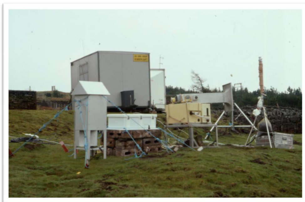
8 - Equipment monitoring atmospheric pollutants at Moor House in 1993. This was part of an international campaign organised by UMIST and the Institute of Terrestrial Ecology, Edinburgh.
